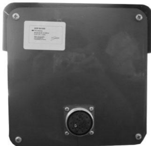
Socket for thermal camera connection
