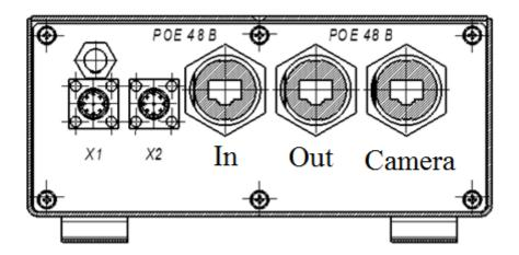
X1, X2 – to connect security sensors, floodlight and external power supply.
