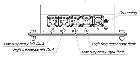
X1–X4 – sockets for connecting sensing elements
