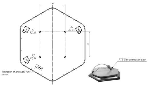
Connectors X1-X3 are equivalent and used to connect devices - STS-507communication controller and battery unit.
