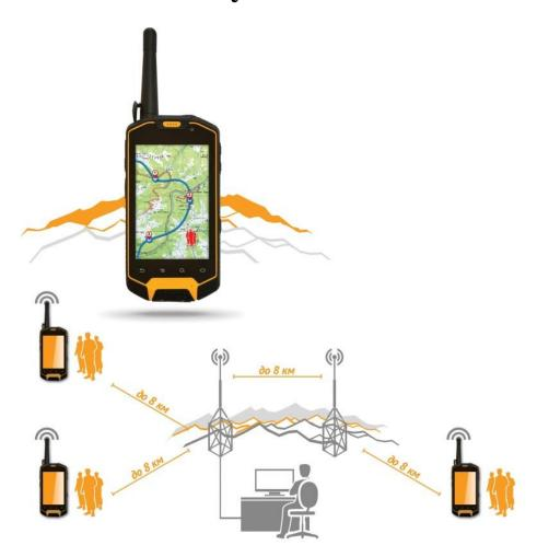
"Unicom-1" is intended to provide communication between patrolling squads and control and command center.
